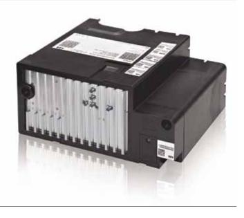
The eVD4 has been designed to fully exploit the potential of the IEC 61850 standard and generic object-oriented substation events (GOOSE) technology, including the horizontal high-speed relay-to-relay communication, by means of an inter-panel bus. However, when required, a traditional point-to-point hard-wired connection to the RBX615 relay is possible through 12 digital inputs and eight digital outputs in the plug.
