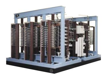
Both the converter and the motor were assembled on site. The converter was shipped from ABB in Turgi, Switzerland, in four pre-assembled units as shown above. The 365-ton motor manufactured by ABB at their works in Birr, Switzerland, was shipped in 3 major pieces (rotor, lower and upper half of stator), with the coolers and accessories shipped and installed separately. Final motor connections were done by ABB in Richmond, Virginia.
