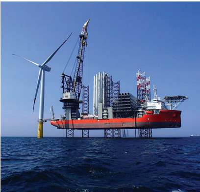
World's biggest wind turbine installation vessel: Pacific Orca – Swire Blue Ocean
