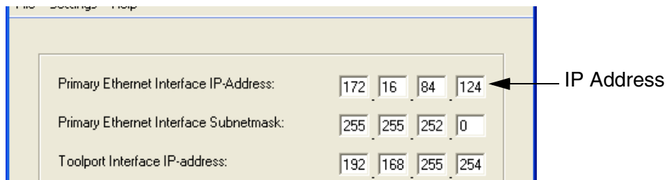
Figure 55. IP Config window for setting unique IP address
