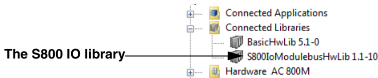
Figure 44. The new S800IO library has been connected to the controller
