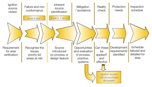
The ATEX process requires operators to consider hazardous area management as a 'cradle to grave' concept consisting of appropriately assessed zoned areas to be at a minimum followed by correct equipment selection and management systems to ensure ongoing compliance.
