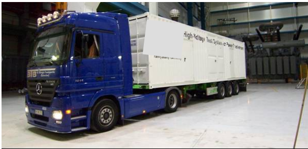
Fig. 8 Mobile High Voltage Test System built on a 40' container arrive to the site for test
