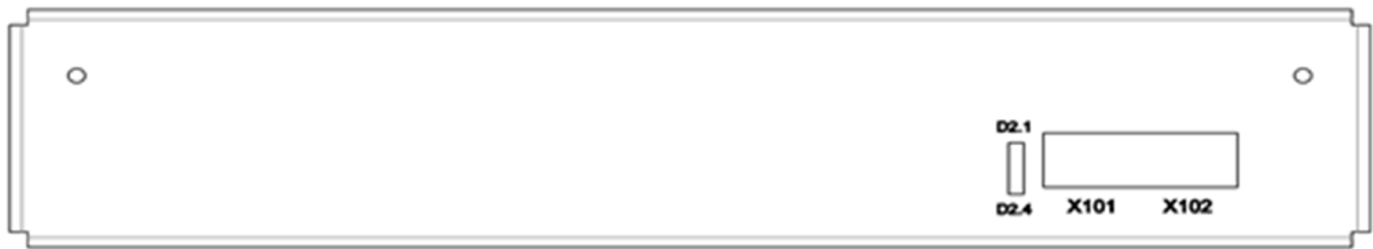
Figure 10. SAM600-VT module fiber optical Ethernet side view
