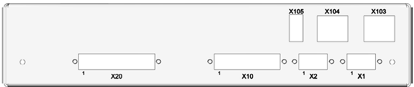
Figure 9. SAM600-VT module electrical Ethernet side view
