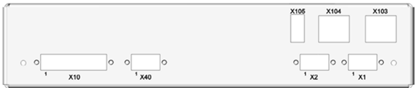
Figure 11. SAM600-TS module electrical Ethernet side view
