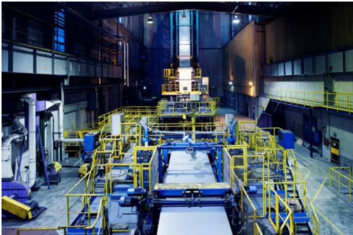
Fig. 1: Hot-dip galvanizing; source: voestalpine
