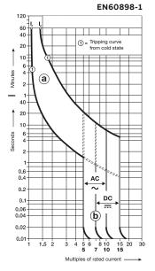
Trip characteristics: C Thermal trip 1.13...1.45 x I, acc. to EN60898-1 Thermal trip 1.05...1.3 x I, acc. to EN60947-2 Electromagnetic trip 5...10 x I, AC 7...14 x I, DC Calibration temperature 30°C
