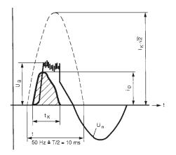
$I_{\kappa} \cdot \sqrt{2}$ = peak value of prospective short-circuit current = Max. peak let through current of circuit breaker S 400 Ŭ,
