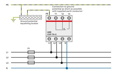
Auxiliary switches and signal contacts
