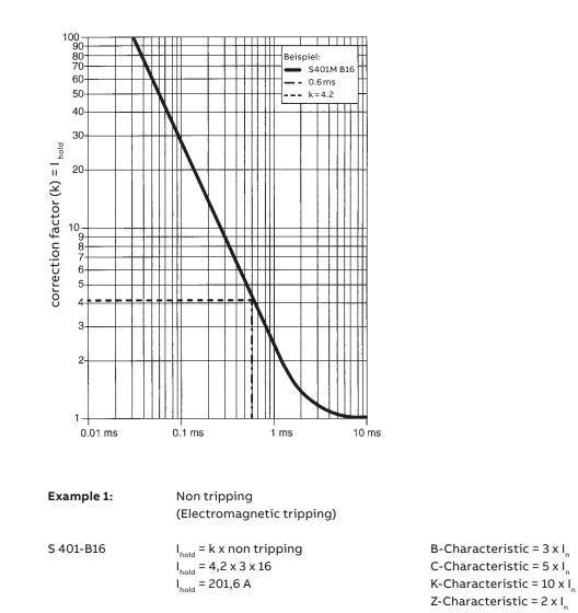
The MCB S 401-B16 hold is keeping by an Impulse of 0.6 ms up to a current of 201.6 A.
