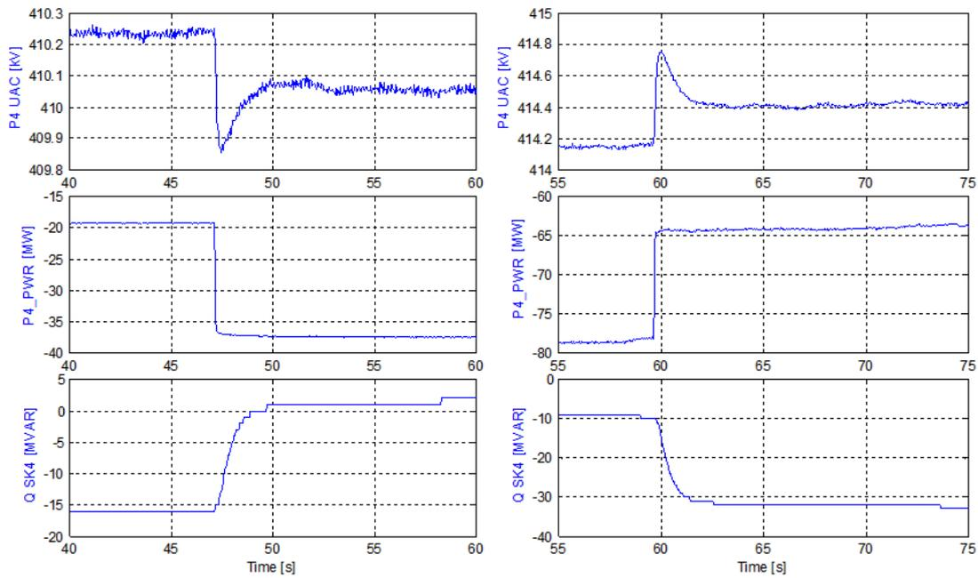
Figure 5: Connection (left side) and disconnection (right side) of load from the islanded grid
