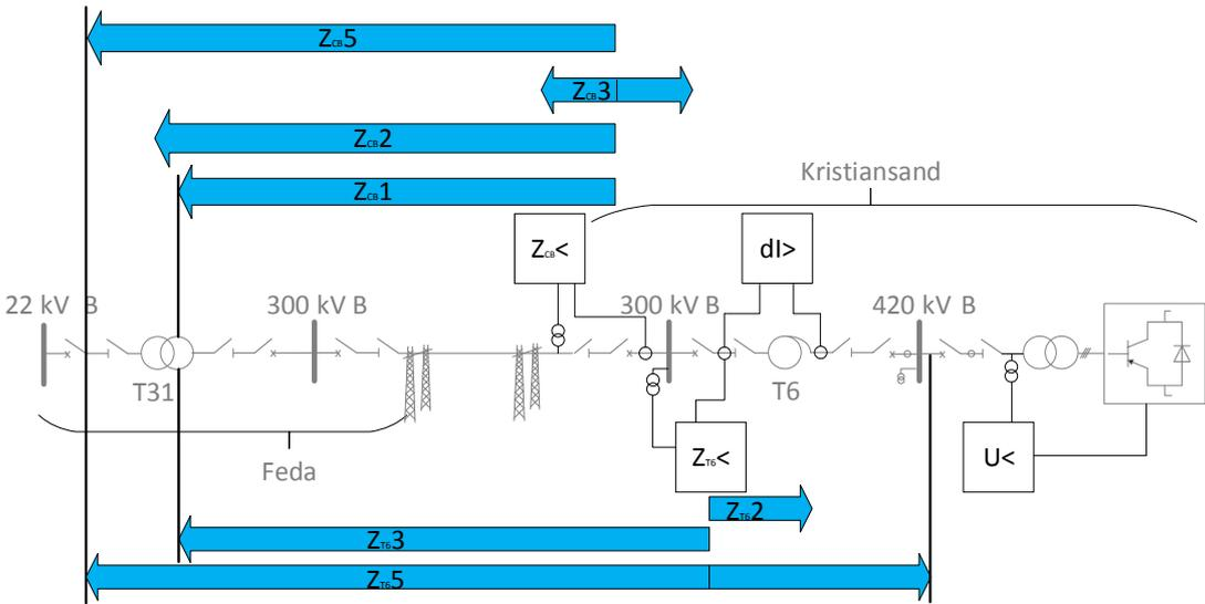
Figure 3: Changes in protection settings for the black-start test, distance relays shown at top of the figure located at the 300 kV breaker bay in Kristiansand, the distance relays shown at the bottom of the figure located at the 420/300 kV transformer in Kristiansand
