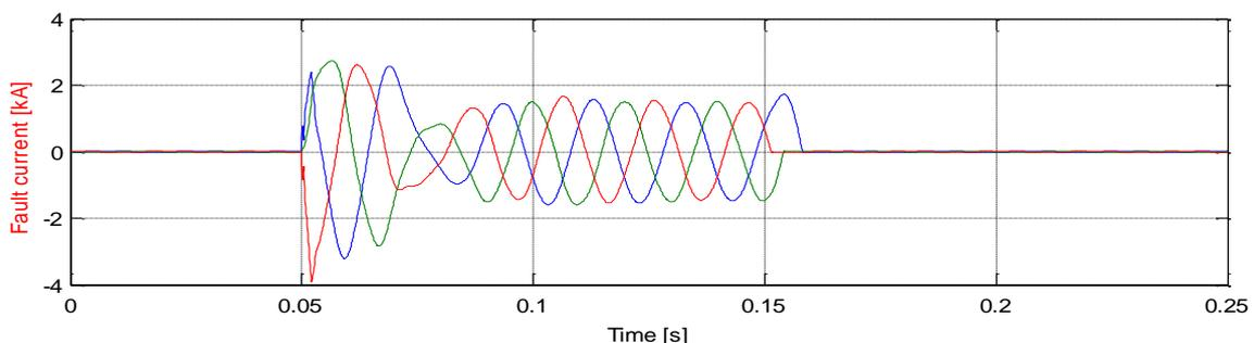
Figure 2: PSCAD simulation of fault current at three phase fault on the Kristiansand 420 kV bus
