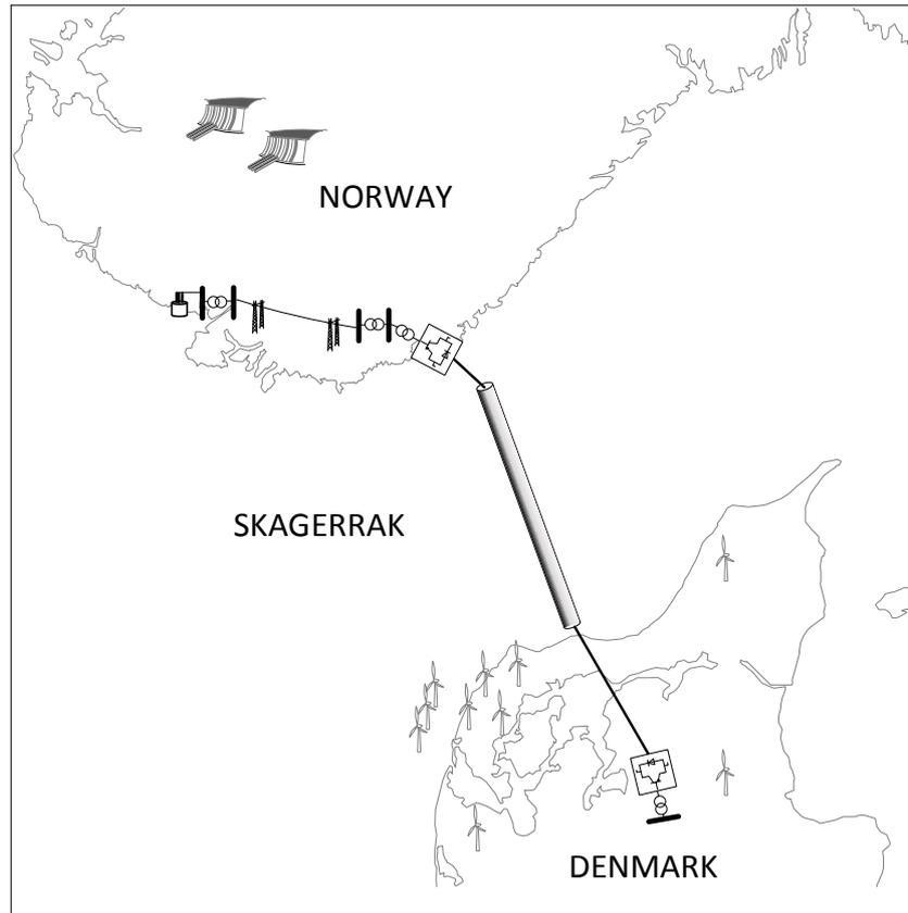
Figure 1: Skagerrak 4 HVDC Link with Black-start test grid
