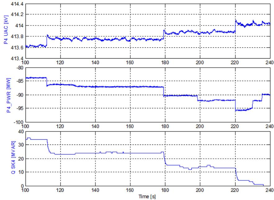
Figure 6: Connection of capacitor banks at Eramet 24 kV busbar
