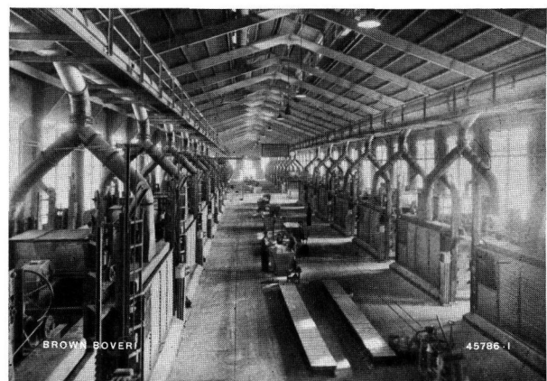
Fig. 1. — Furnace room in an aluminium works with Soederberg furnaces each of 32,000 A.
