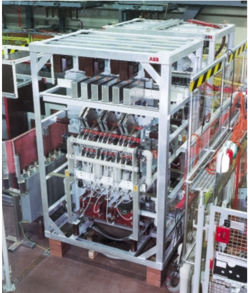
High-power IGCT inverter module, for which a design with 6 series-connected devices is normally chosen. Each 4.5-kV device of the module can be loaded with a maximum of 3 kV DC. It is equipped with reduced du/dt snubbers of a simple RCD type. The gate-drive supply is realized with special isolation transformers.
