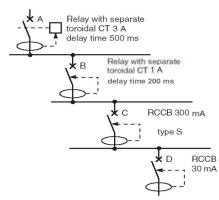
The time delay option is allowed to establish selectivity between upstream and downstream devices as shown below. In the SLD shown, All 4 circuit breakers are coordinated to ensure proper selectivity. Circuit breakers A&B are with MRCD's (Earth leakage relays). Circuit breaker C is selective type and circuit breaker D is with no time delay.
