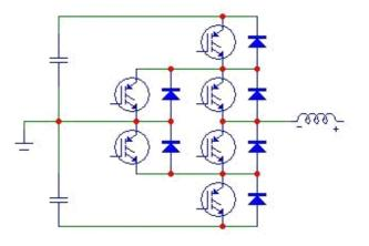
*Figure 1: Three-level converter principal circuit diagram for one phase. Each IGBT / diode symbol is in reality made up of more than 150 presspack IGBT modules in Cross Sound Cable and Murraylink.*
