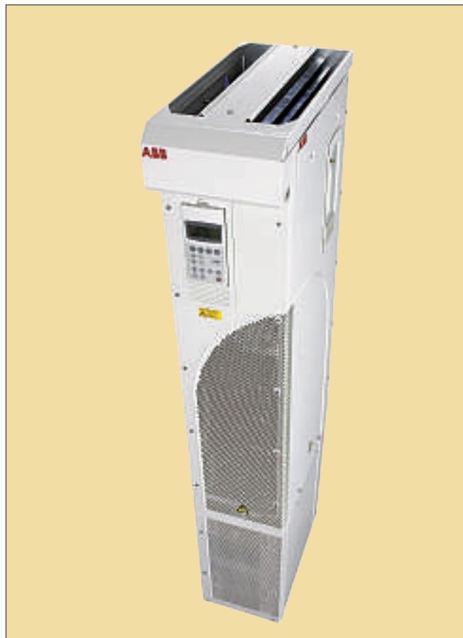
The ACS800-02 drive, available in the 90 - 150 kW power range, is only one-sixth the size of comparable drives from other manufacturers. The reduction in size has been achieved using new, advanced electronic components in combination with the latest insulation and cooling technologies.
