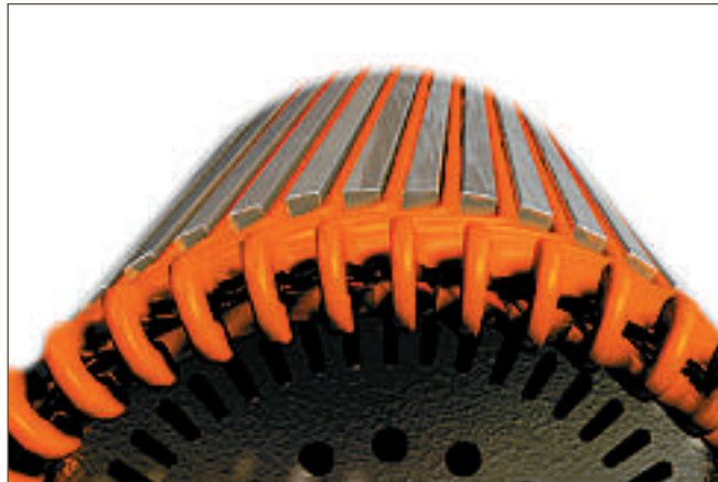
4 The armature coils are skewed for smoother running at low speeds and less noise.
