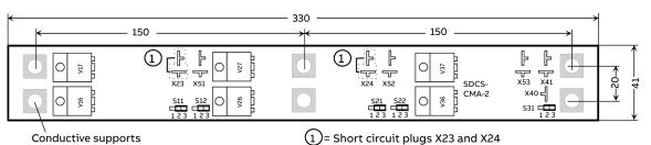
Jumpers S11 ... S31 and short circuit plugs X23, X24 are shown at factory settings
