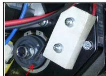
Figure 6. Cam Orientation when charged
