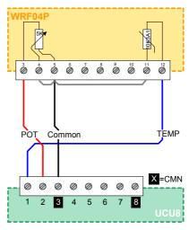
te: To avoid self-heating, which can affect the accuracy of measurement, the wire current should not exceed 1mA.
