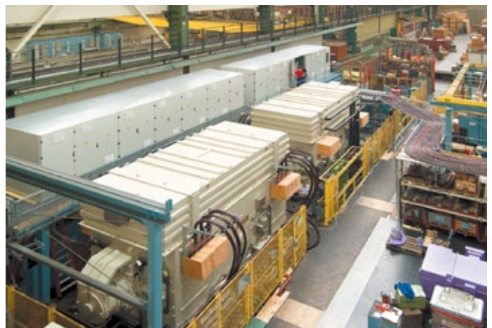
Back-to-back test set-up
