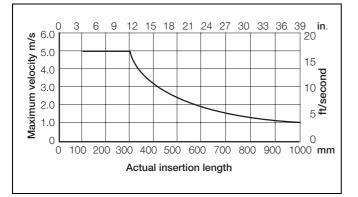
\*The graph is intended as a guide only. It is not possible to be definite as there are many effects which cannot be allowed for in such circumstances. For example, pipe vibration, fluid vibration due to pump noise, position of cable, orientation of probe entry, etc.
