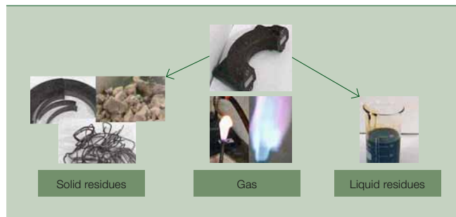
2 Products from pyrolysis of used epoxy product
