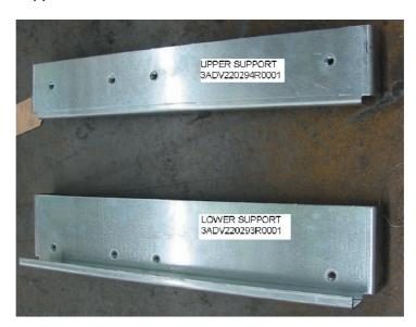
The upper and lower mounting rails should be fixed into the cabinet with a distance of 1520 mm between their lower edges. If your cabinet's grid of fixing holes in the mounting rail does not allow this distance, you may vary the distance by some mms due to the elongated fixing holes in the panel.
