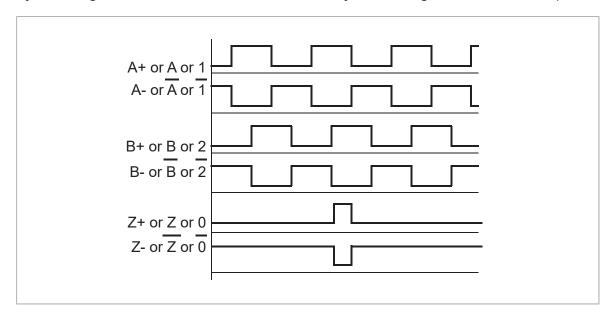
The encoder output channel that leads when the drive runs Forward should be connected to FEN-01 input A, the output channel that trails to FEN-01 input B.
