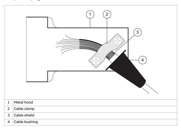
Note: Do not route the encoder cables parallel to power (e.g. motor) cables.
