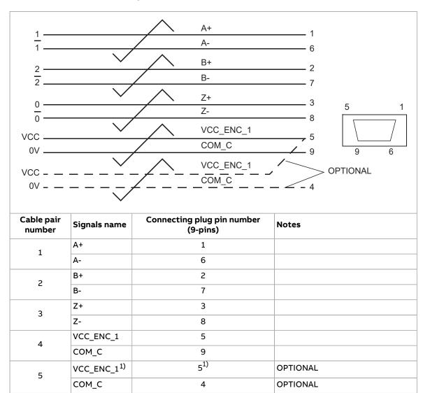
$<sup>^{1)}</sup>$  Two wires soldered to the same pin.
