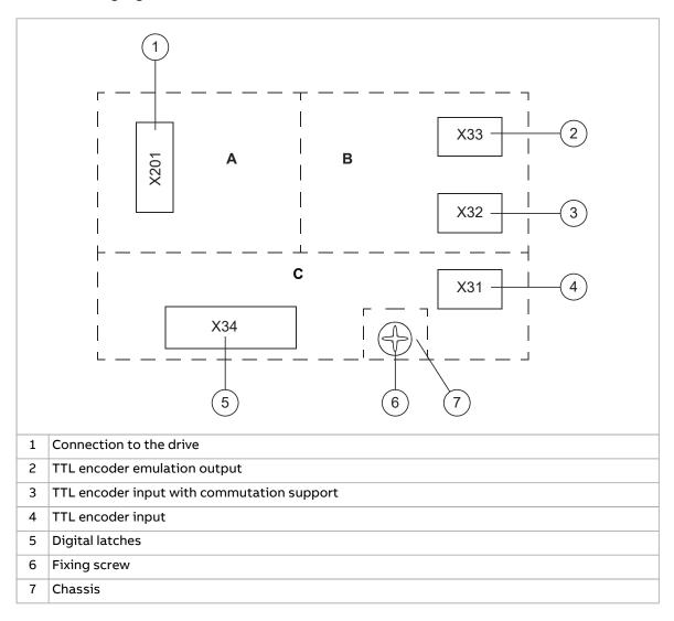
The shields of sockets X31 and X32 and plug X33 are connected to chassis. The fixing screw connects the chassis to ground.
