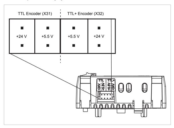
**Note:** If an external power supply is used, the appropriate jumper must be removed.
