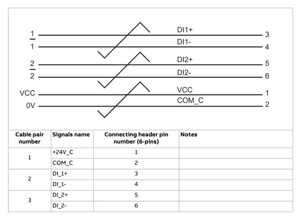
Note: Do not route the encoder cables parallel to power (e.g. motor) cables.
