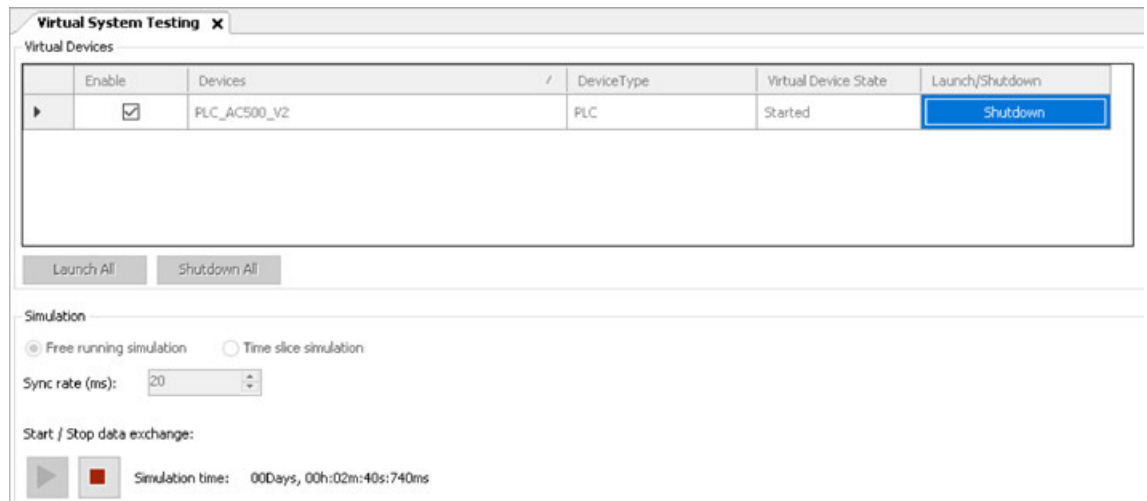
Fig. 1178: Free running simulation
