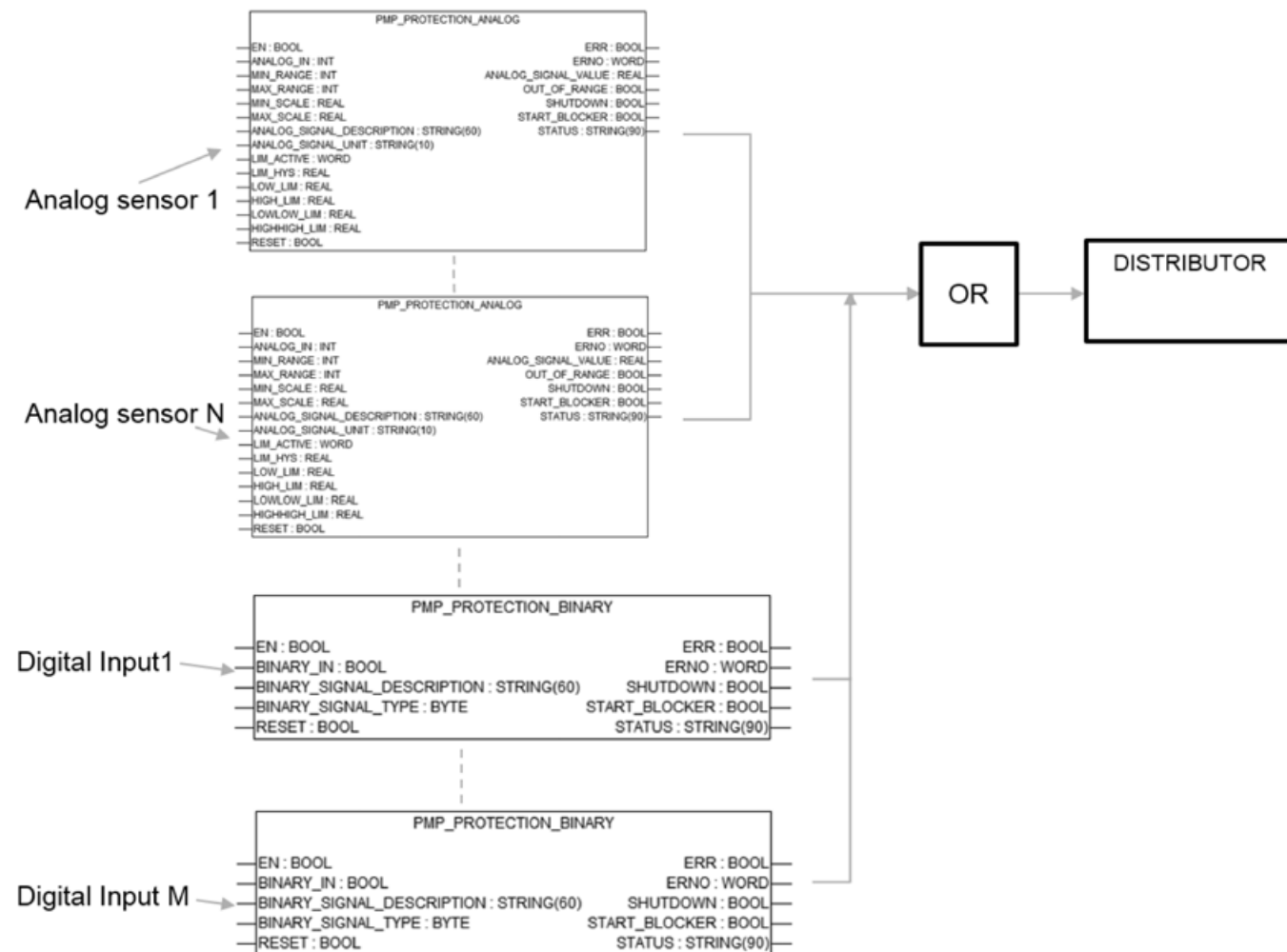
Fig. 717: Analog/Digital FB - process specific protection
