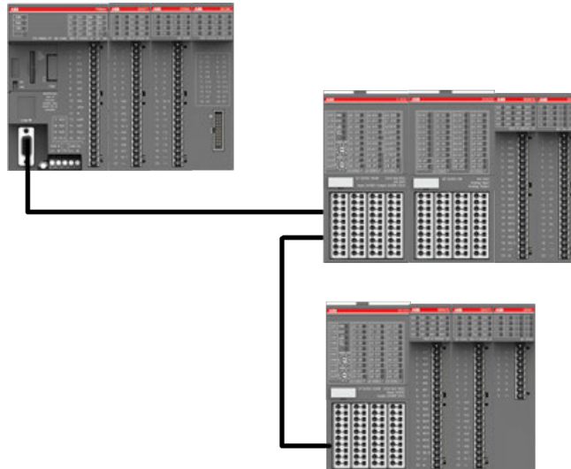
Fig. 726: I/O modules (S500-eCo) connected to a AC500-eCo processor module via CS31 bus
