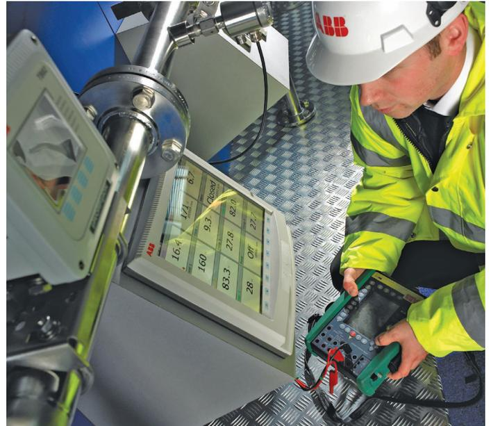
Fig. 6: Checking recorded process data can help to detect signs of deteriorating instrument performance
