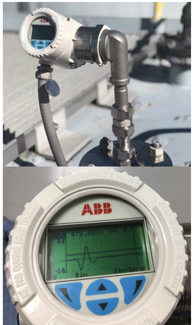
Clean strong noise free signal in an LMT10 with flexible probe even at 478.88"
