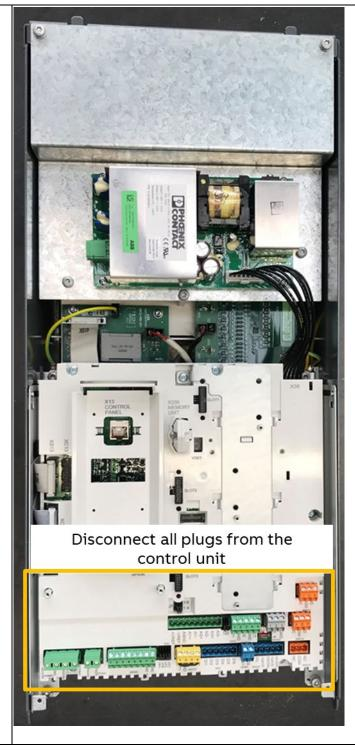
4. Remove the grounding/holding screws from the electronic unit.
