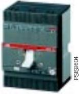
**S2D 125**  $I_n (40\text{ }^\circ\text{C}) = 125\text{ A}$   $I_{cw} (1\text{s}) = 2.2\text{ kA}$   $I_{cm} (415\text{ V}) = 3.1\text{ kA}$
