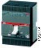
**S2B 160**     $I_n (40\text{ }^\circ\text{C}) = 160\text{ A}$      $I_{cu} (415\text{ V}) = 16\text{ kA}$
