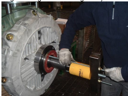
Removal of seals with puller
