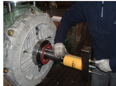
Removal of seals with puller
