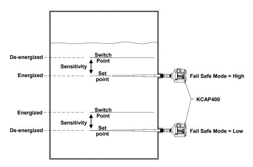
Setting the Fail Safe to High on the Upper Switch will cause the relays to de-energize when the sensed capacitance reaches the Setpoint plus the Sensitivity. The relays will energize after the sensed capacitance moves down past 1/3 of the Sensitivity plus the Setpoint.
