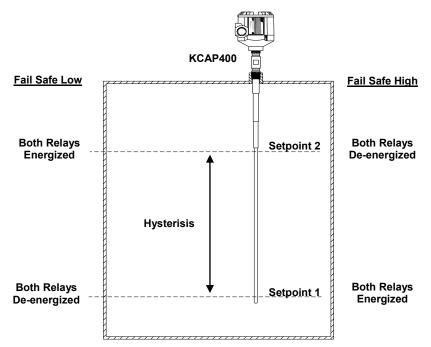
If the KCAP400 is changed from Dual Setpoint Mode to Pump Control Mode, the Setpoints and the Time Delay will remain at their current settings. The Sensitivity / Hysterisis will become the difference between the switches.
