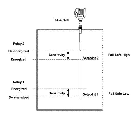
If the KCAP400 is switched from Single Setpoint Mode to Dual Setpoint Mode, Setpoint 2 will become active, along with the stored value for its' Fail Safe Mode. Setpoint 2 will have the same Sensitivity and Time Delay as Setpoint 1. If Setpoint 2 has not been calibrated, the default values from stored memory will apply.
