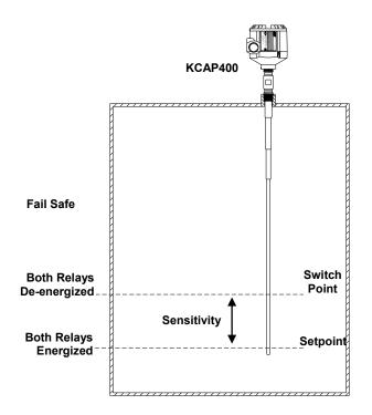
If a KCAP400 is switched from Dual Set Point to Single Setpoint Mode the value of Setpoint 1 will be maintained, along with its Fail Safe Mode, Sensitivity, and Time Delay. Setpoint 2 will, in effect, be turned off and its' settings will be stored in memory.
