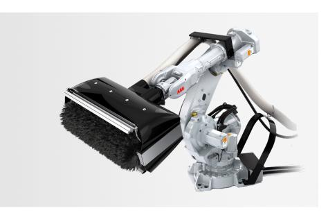
The FeatherDuster system advances vehicle paint lines by replacing purpose-built "tack off" machines with robotic technology that is incredibly flexible and built on well-established standards to achieve higher quality, efficiency and ease of use.
