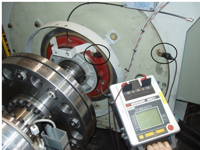
Figure 34 Measuring the insulation resistance of a roller bearing
