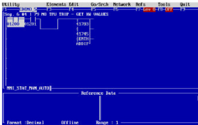
Figure 84 – If No TPU Trip Calculate KW Values Prior To Trip For Later Loading Calculations For Bus Line Sectionalizing Calculations
