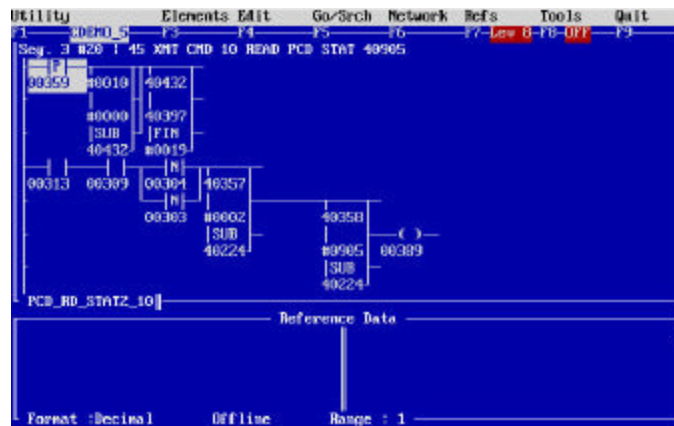
Figure 49 – Segment 3 Network 20 – Read PCD Status Information Or FIFO Instruction Load.
