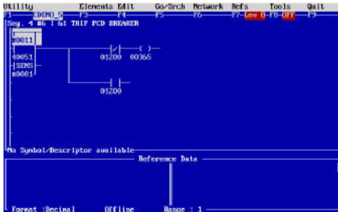
Figure 66 – Segment 4 Network 6 - MAGELIS PCD Manual Trip Pushbutton Logic
