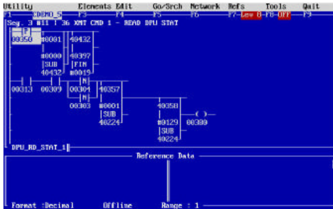
Figure 40 – Segment 3 Network 11 – Read DPU Status Information Or FIFO Instruction Load.
