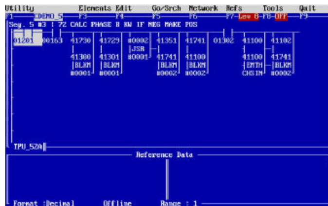
Figure 77 – Segment 5 Network 3 - Calculate KW For Phase B
