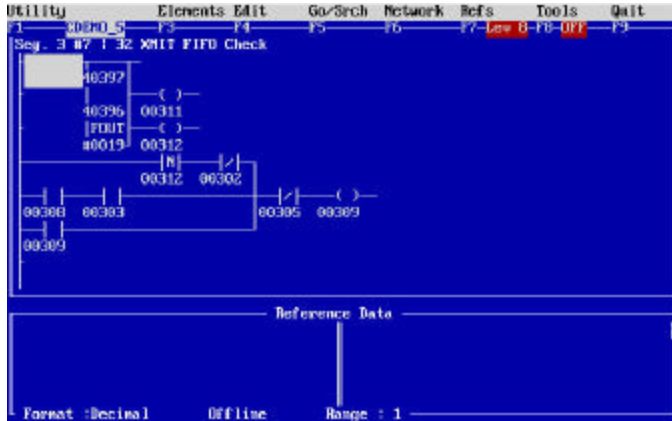
Figure 36 – Segment 3 Network 7 – FIFO Empty/Full Notification Logic
