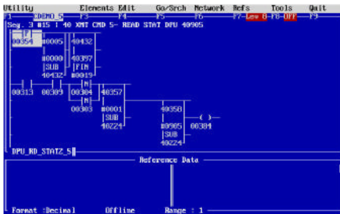
Figure 44 – Segment 3 Network 15 – Read DPU Status Information Or FIFO Instruction Load.
