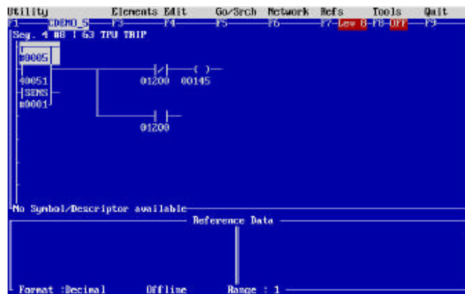
Figure 68 – Segment 4 Network 8 - MAGELIS TPU Manual Trip Pushbutton Logic
