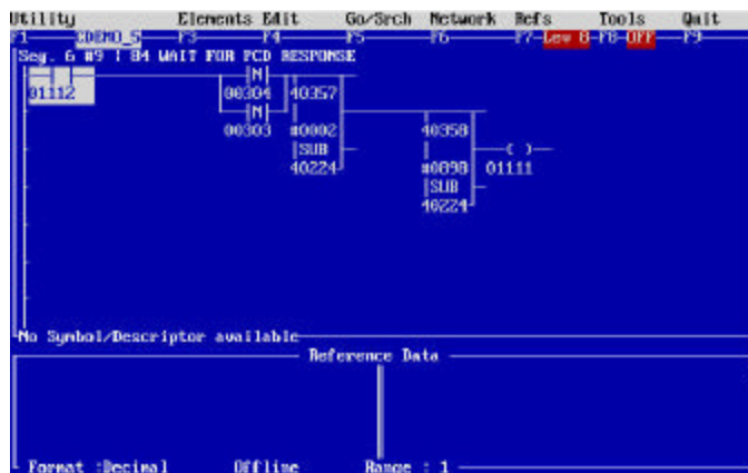
Figure 89 - Segment 6 Network 9 - Wait For PCD Response To Breaker Action
