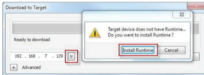
2. Download a project with PB610 Panel Builder 600 to install the Runtime. When you download a project the Runtime is automatically installed if needed. See *“Transferring the project to HMI device”* for details.
