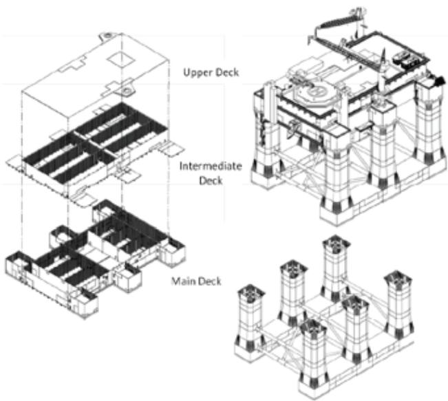
Fig. 2 Modularization of a gravity based structure platform. The topside structure is the same for all concepts, whereas the substructure is sized for water depth and power rating.
