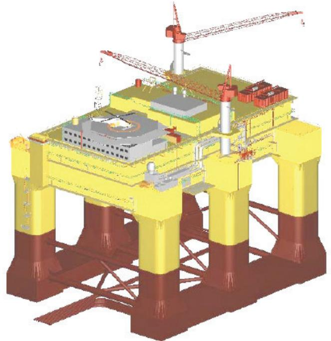
Fig. 1 A 3-D model of the GBS platform for Dolwin2.
