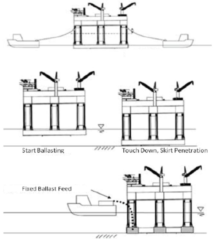
Fig. 3 Transportation, installation and positioning of gravity based structure.
