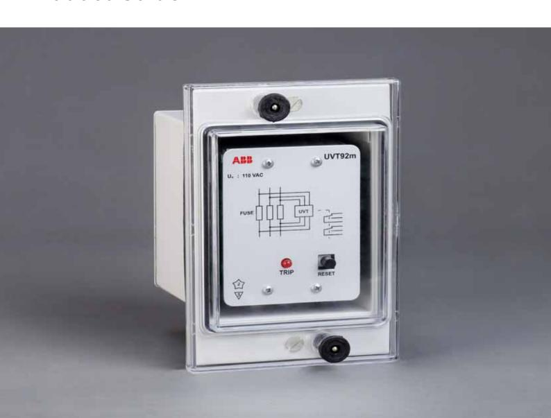
UVT92m is a high speed static relay intended for continuous monitoring of fuses against blowing out or inadvertent removals. This relay can be used for one, two or all three phase fuse failure detection. The plug-in socket type design for terminals, supports ease of installation and maintenance.
