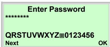
4. Enter the corresponding password (see Chapter "Selecting and changing parameters"). There is no factory default for the password. You can switch to the configuration level without entering a password. The selected access level remains active for 3 minutes. Within this time period you can toggle between the process display and the configuration level without re-entering the password.
