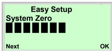
43. Use to start automatic balancing of the zero point for the system.
