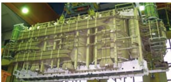
Phaseshifter Activepart, 450 MVA, 138 kV, shift angle 50 degree.
