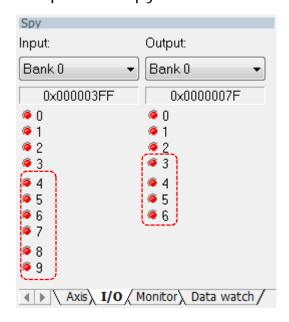
4 to 9 of *Input Bank O* are OPT-SIO-1 extended DIN4~DIN9, and 3 to 6 of *Output Bank O* are OPT-SIO-1 extended DOUT3~DOUT6.
