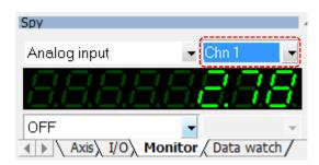
Analog input Chn1 (as shown above) is the analog input (AIN1) of the OPT-SIO-1.
