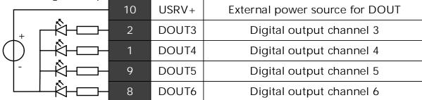
0V...30V DC source, 100mA nominal load, 300mA PTC Resettable Fuse
