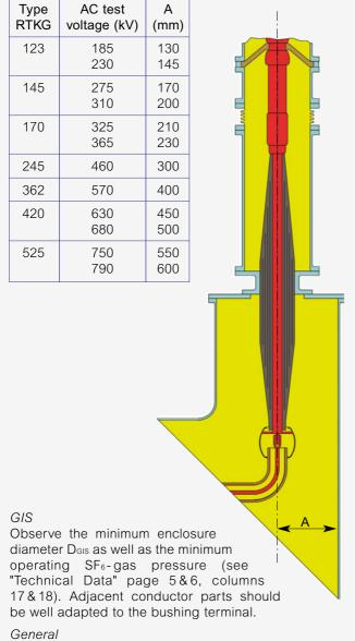
Because the bushing is completely dry it can be operated vertically or horizontally or in any position.
