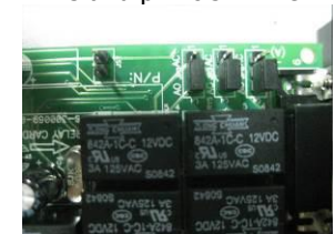
Fig. 5 AO and AC silk printings indicates each 3-pin connector status To achieve ACTIVE CLOSE dry-contact signal, the jumper should connect the 2 pins(Pin1&2) as shown in Fig. 6.
