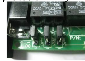
Fig. 7 Jumper setting for ACTIVE OPEN
