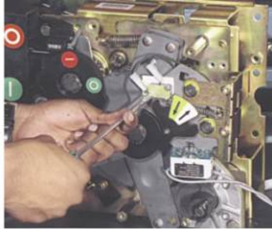
Unscrew the microswitch fixing screws
