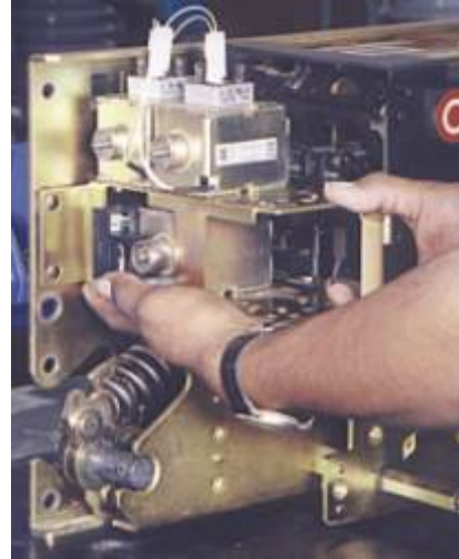
Withdraw the release group mount from the front of the operating mechanism. For assembly, proceed in the reverse order.
