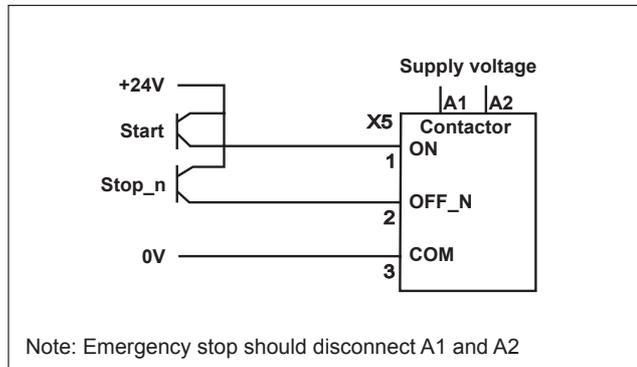
When used with transistor outputs the wiring can be done according to the following diagram.
