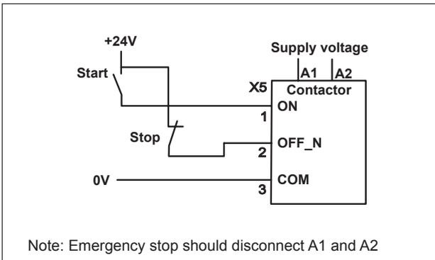
When used with switches the wiring can be done according to the following diagram.
