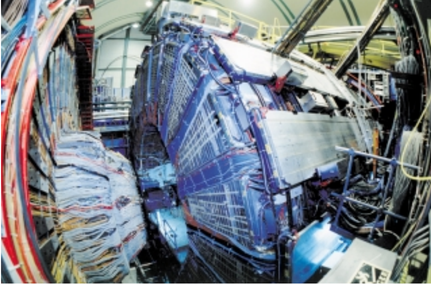
Partially opened DELPHI particle detector. On the right is the main section with \mu on calorimeters, on the left the end-plug with some of the cabling for the 1 million data points. 2
