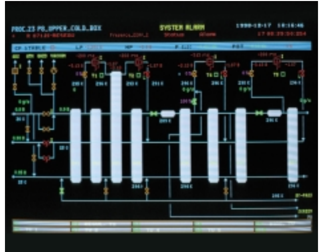
Upper cold box, in which turbines expand the helium, thereby cooling it from 300 K to 20 K.
