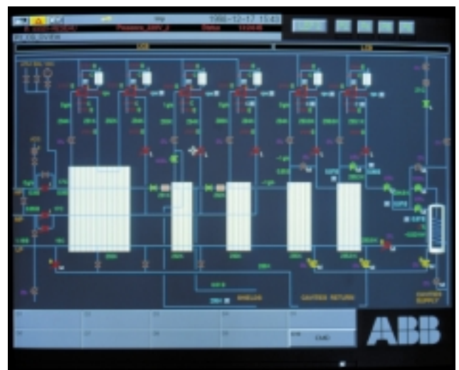
Cryogenic installation (upper and lower cold box). The helium is liquefied from 20 °C at 20 atm to 4.2 K by means of expansion turbines. 4
