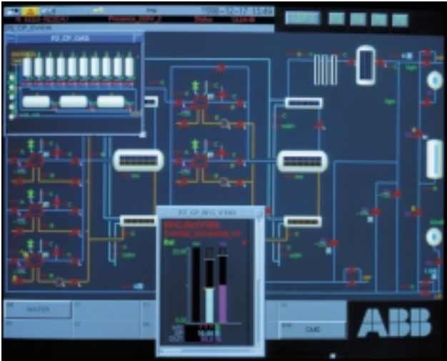
Compressor stage of the helium liquefier at LEP site 2. Five parallel compressors belonging to the low-pressure section are shown on the left. The inset shows tanks holding helium gas in reserve at normal temperature.
