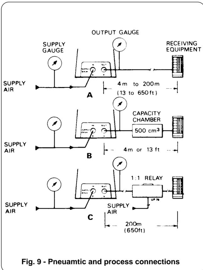
Fig. 9 - Pneumatic and process connections
