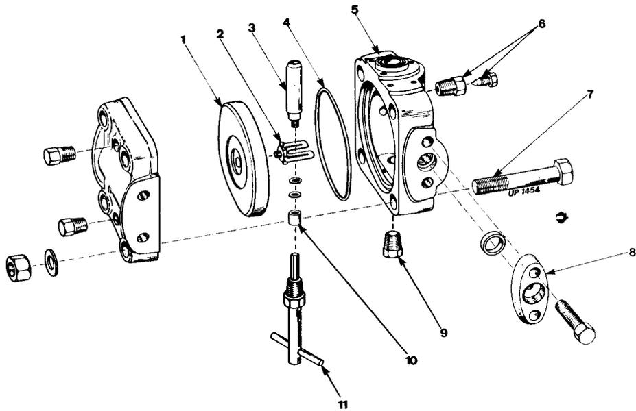
Fig. 1A - NBC model exploded view of measuring element
