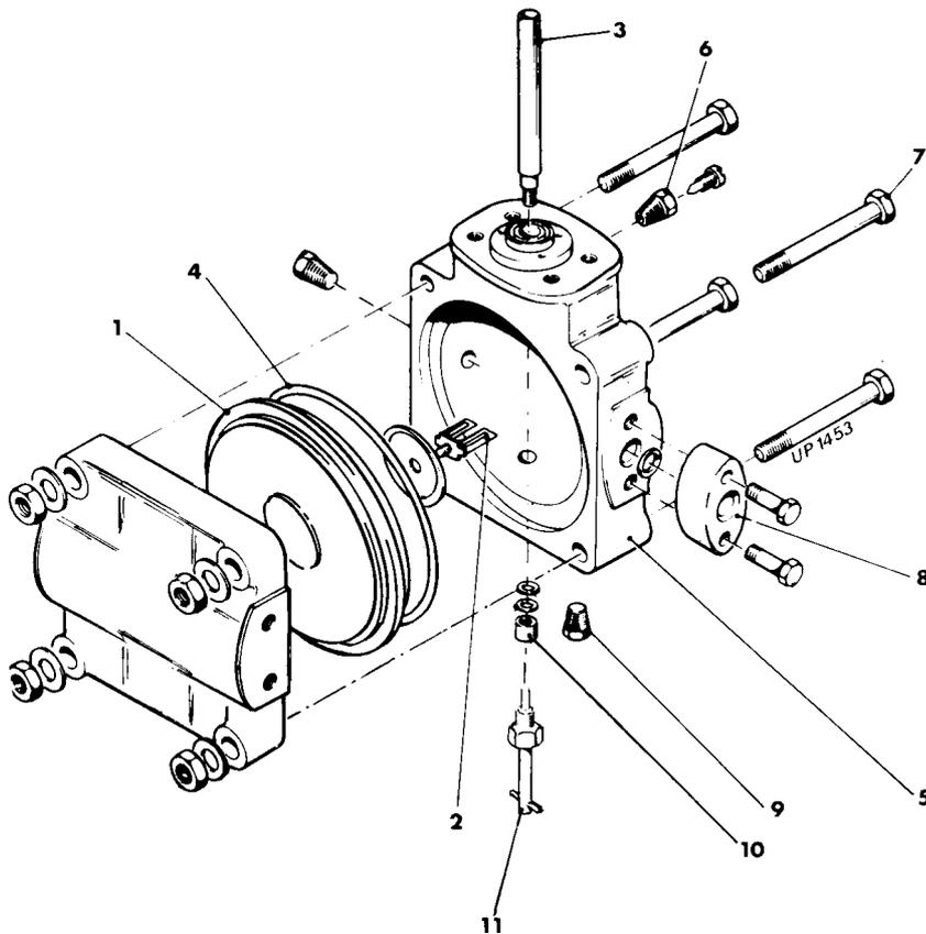
Fig. 1B - NBD model exploded view of measuring element
