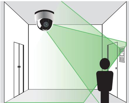
Camera module integration. When video outdoor station is integrated with an analog camera, the field of vision and monitoring range will be significantly enlarged. In addition, residents are free to switch between the inbuilt camera on outdoor station and the additional analog camera for surveillance purpose through cyclic selection among all outdoor stations, no matter in standby or during video conversation with visitors.
