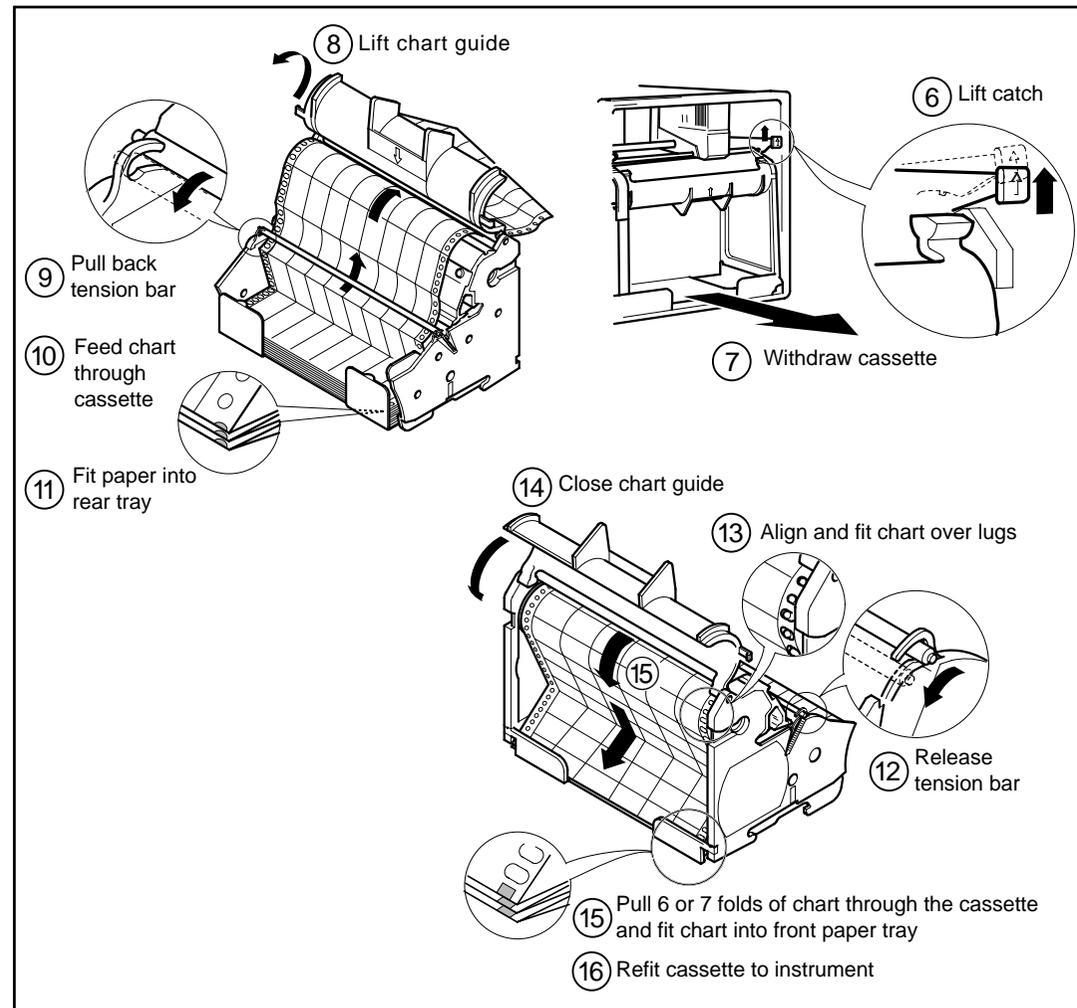
**Caution.** Once chart loading is complete, ensure the correct chart type is set in the **Chart Control Configuration Page** – see Section 5.3.1 in the User Guide.
