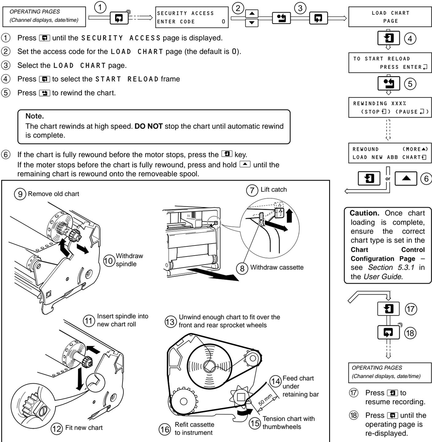
**Caution.** Once chart loading is complete, ensure the correct chart type is set in the **Chart Control Configuration Page** – see Section 5.3.1 in the User Guide.
