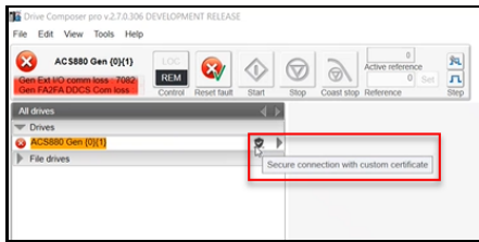
Figure 40. Secure connection with custom certificate
