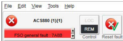
Figure 148. FSO configuration: FSO general fault due to configuration state
