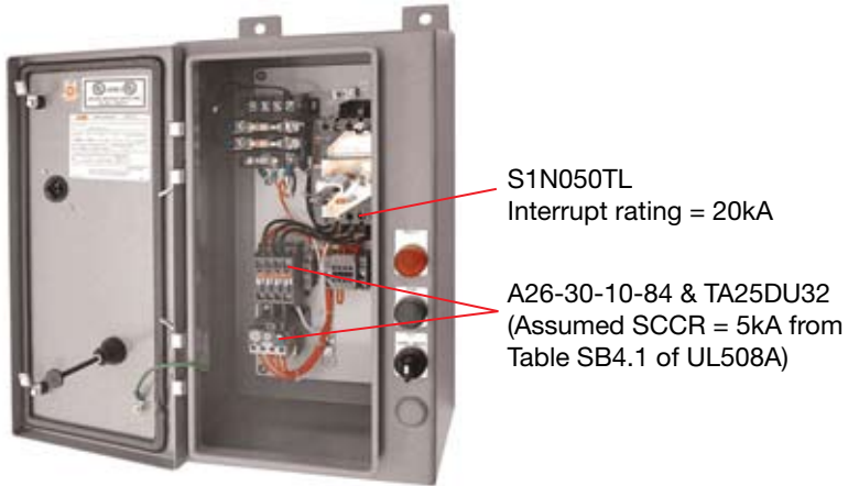
Fig.2 - Example #1, Industrial Control Panel
