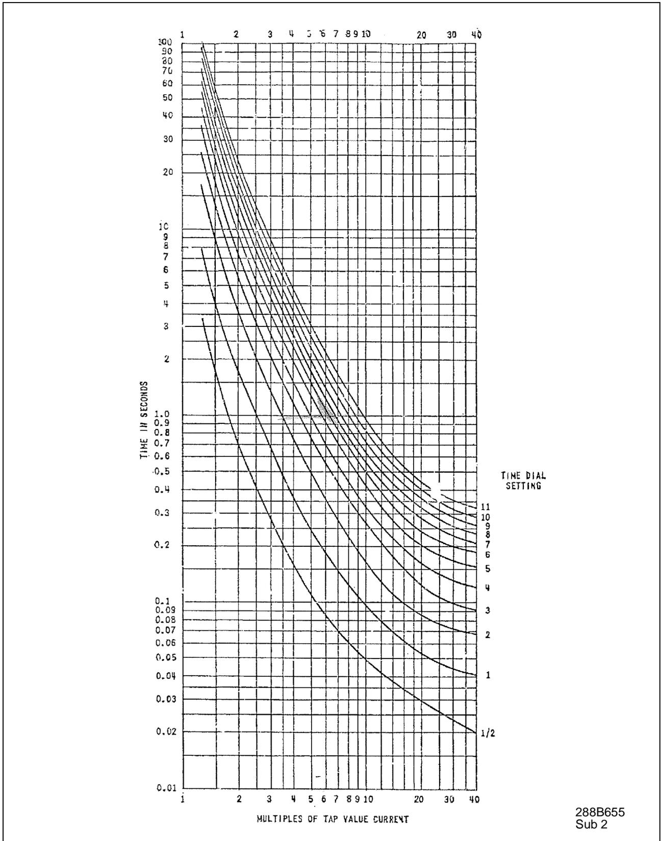
Figure 9: Typical Time Curve of the Type CO-11 Relay
